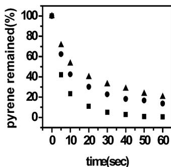
**Figure 5.** Release kinetics of pyrene from multilayer films of PDPA and PS<sub>21</sub>-PAA<sub>157</sub> micelles: (■) 0.5 M NaCl solution, (●) 0.1 M NaCl solution, (▲) 0.01 M NaCl solution.
