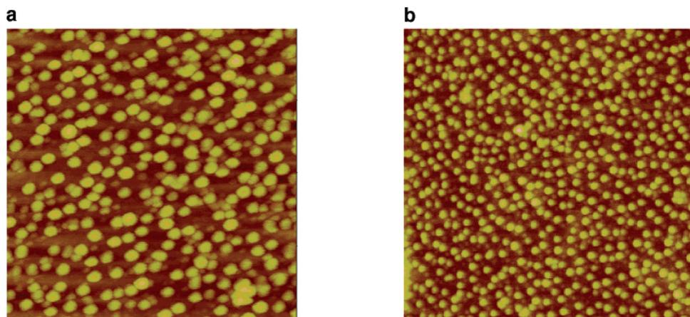
**Figure 6.** In-situ AFM images of 1-bilayer PDDA/micelles film before (a) and after (b) injection of 0.1 M NaCl aqueous solution into the liquid cell. Scale:  $1.0 \mu\text{m} \times 1.0 \mu\text{m}$
