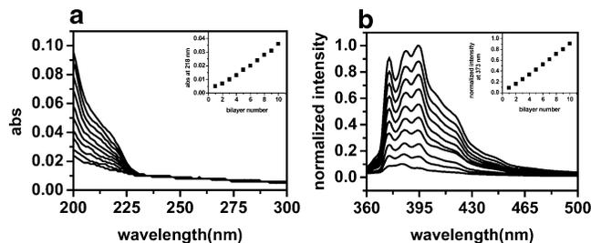
**Figure 1.** UV-vis (a) and fluorescence spectra (b) of a 10-bilayer film of PDDA and pyrene-incorporated micelles of PS<sub>49</sub>-PAA<sub>54</sub>. (inset) Absorbance or normalized intensity versus the number of bilayers.
