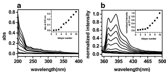
**Figure 3.** UV-vis (a) and fluorescence spectra (b) of a 10-bilayer film of PDDA and pyrene-incorporated micelles of PS<sub>21</sub>-PAA<sub>157</sub>. (inset) Absorbance or normalized intensity versus the number of bilayers.
